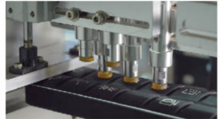
Panel buttons 1.2 million times reliability test
