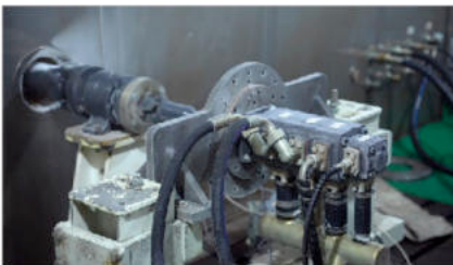
Hydraulic oil pump Low-temperature performance test under -40°C
