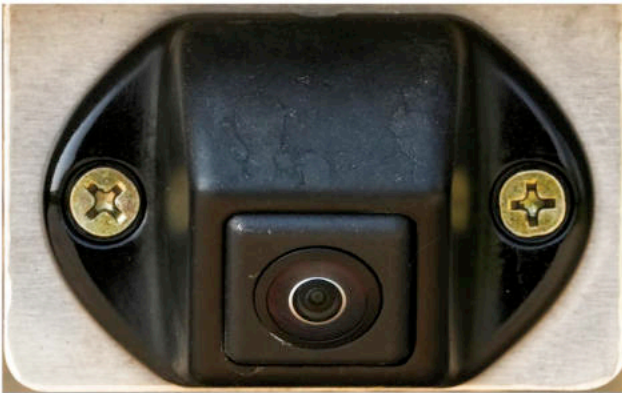
The backup camera helps the driver observe the situation behind the vehicle more clearly when reversing or driving at low speeds.
