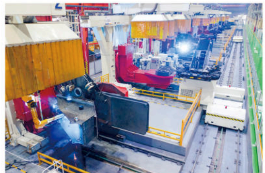
UNMANNED AUTOMATIC WELDING
