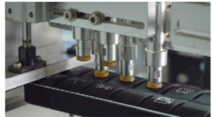
Panel buttons 1.2 million times reliability test
