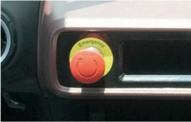
Emergency brake switch: In case of emergency, press this switch to immediately stop all movements of the crane
