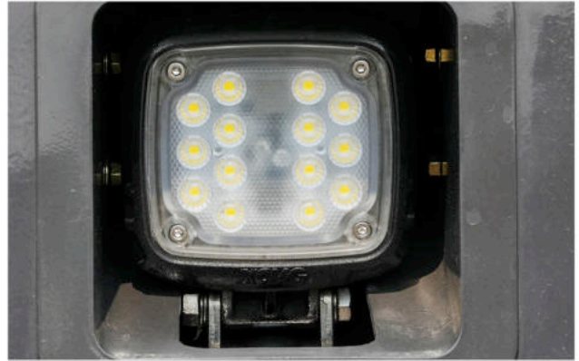
The night lighting device includes work lights of outrigger, turntable and operator's cab, making nighttime operations safer.
